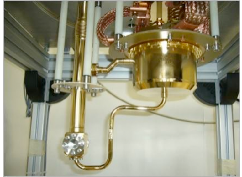
H 2 condenser on GM cryocooler Useful cooling power >25W at 20K Possible high doses >10C/cm 2
